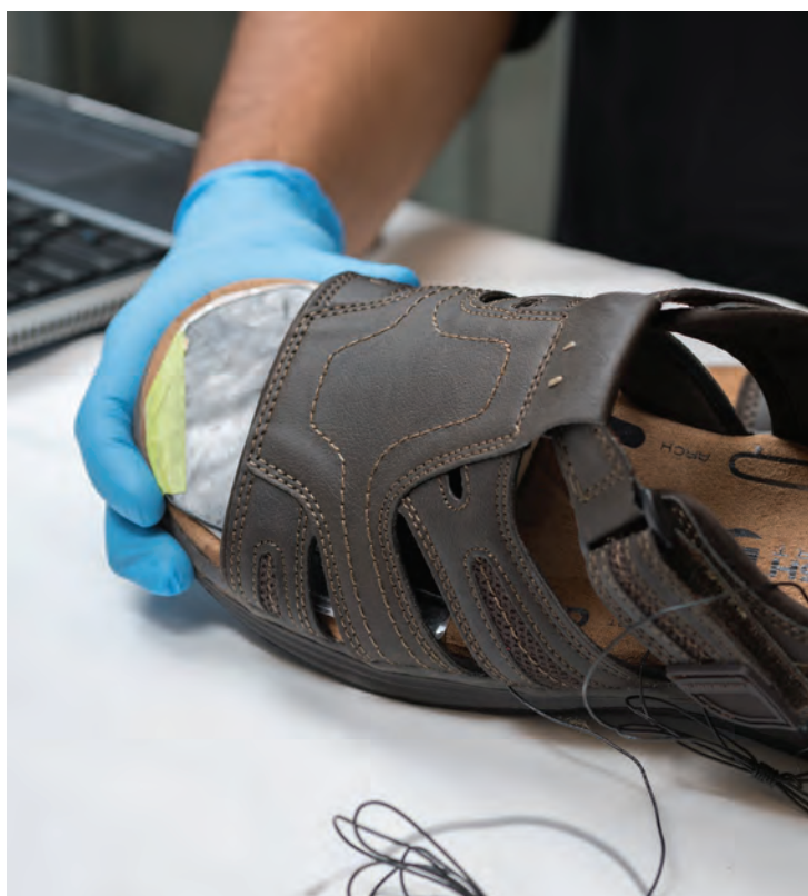
Photos left to right: Doctoral student Sagar Doshi (left) and Erik Thostenson test an elbow sleeve outfitted with one of their novel sensors; Doshi demonstrates how the sensors could be integrated into a shoe to sense pressure on different parts of the foot as a person walks.
