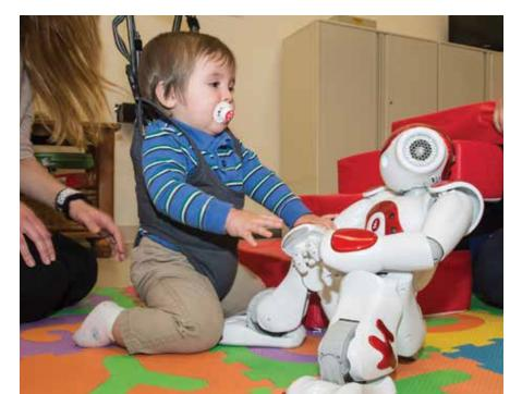
NAO is used in conjunction with a portable harness system that partially supports the weight of special-needs kids and allows them to move freely in an 80-square-foot space, as well as with a network of cameras, sensors and accelerometers that record motion and type of activity.
