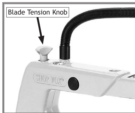
Figure 13. Blade tension knob.
