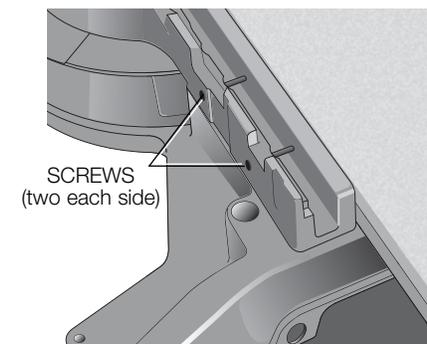
into two pieces. Ensure the screws are tightened properly, otherwise material could loosen and cause injury. Ensure the platform is firmly flat on the table, against the fence, and centered evenly from left to right.
