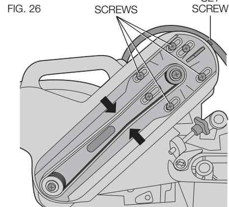
DO NOT use lubricants or cleaners (particularly spray or aerosol) in the vicinity of the plastic guard. The polycarbonate material used in the guard is subject to attack by certain chemicals.
