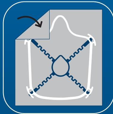
**STEP 2:** Wrap filter material around and into the frame, with spider side down.
