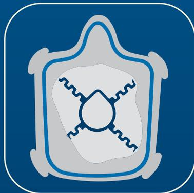
**STEP 3:** Snap retainer hoop into face hoop cage frame.
