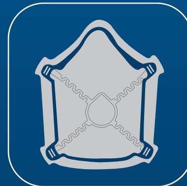
**STEP 4:** Turn mask over and snap strap hoop onto mask. You will feel it snap into the spider hoop.
