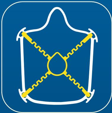
**STEP 1:** Snap tabs of spider into the face hoop to create a cage frame.
