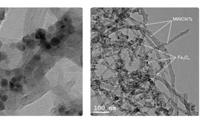
TEM micrographs showing the presence of iron oxide (Fe3O4) spheres on the surface of MWCNTs.
